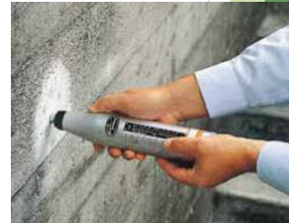
Schmidt Hammer Test.
