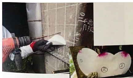
Measurement of carbonation depth
